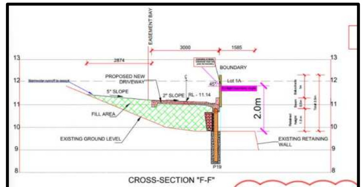
Figure 23: Cross-section F-F along the boundary of Allotment 1A and 17 Chapel Street, showing sunlight breach where the structure exceeds 2m in height.
