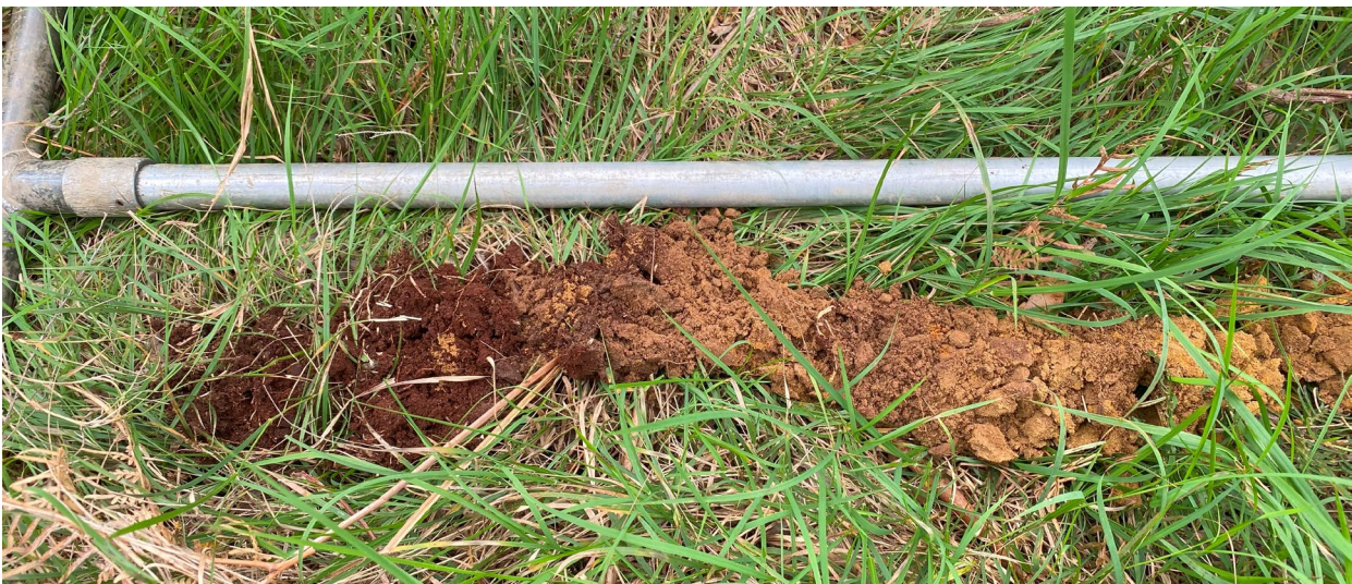
Photograph 1: Showing a soil sample from BH 1, 50mm of slightly moist, brown, sandy topsoil followed by slightly moist, fine, brownish orange then orange sand.
