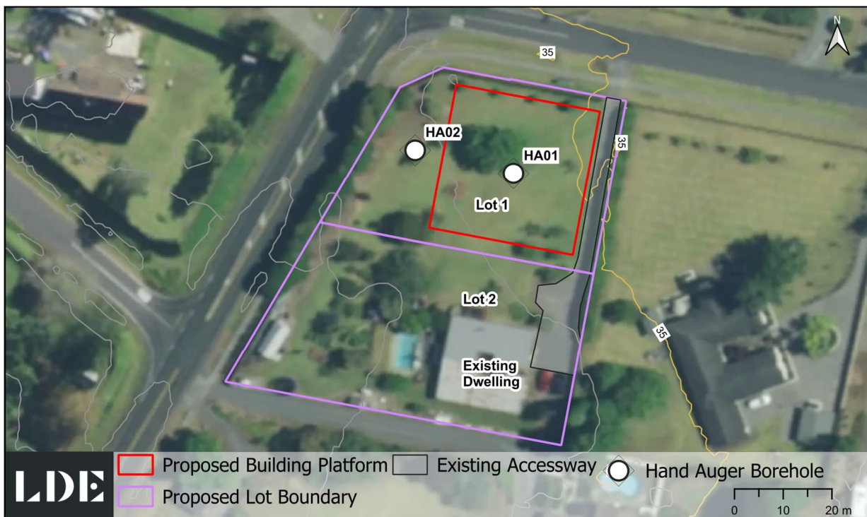
Figure 13: Geotechnical investigation plan.
