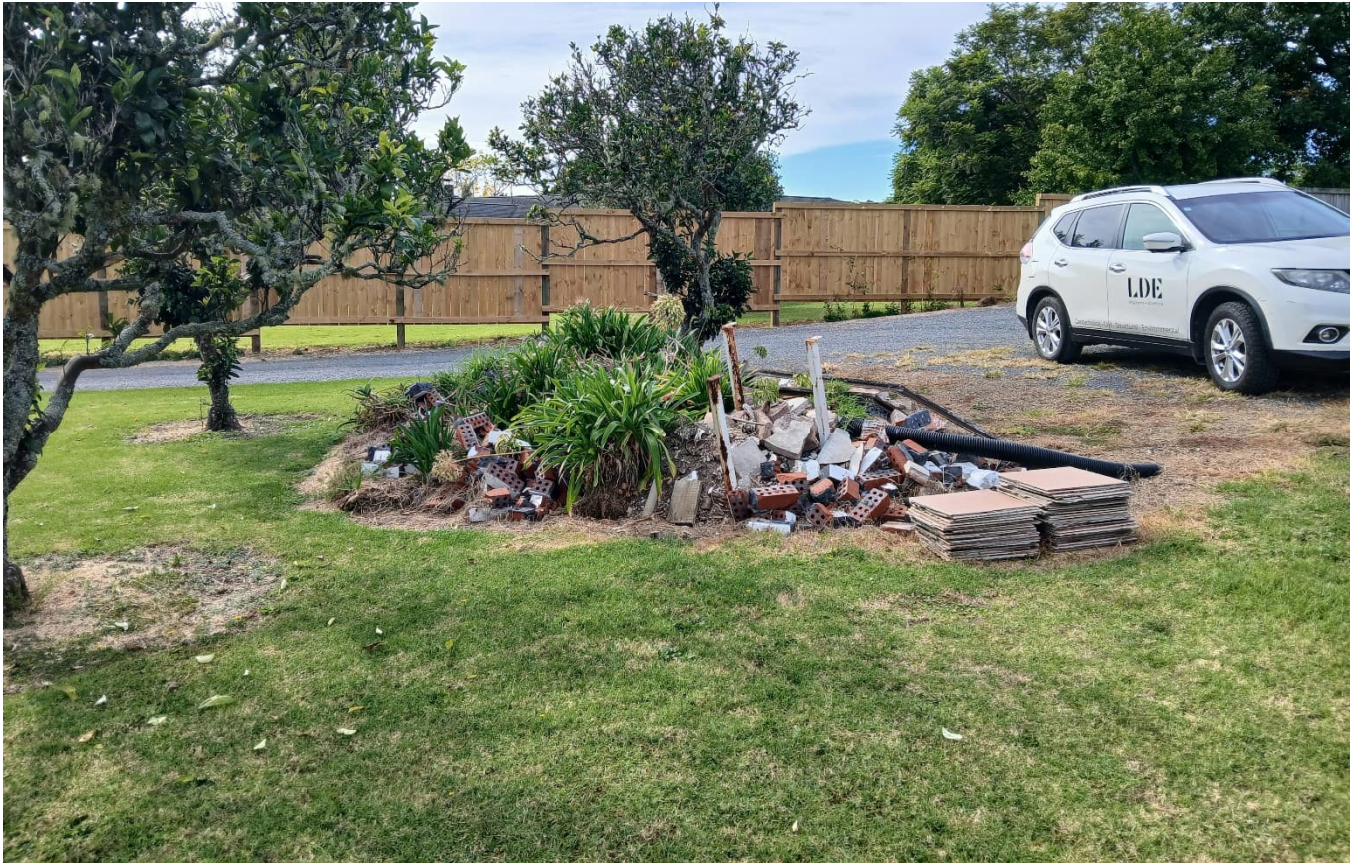
Figure 9. Pile of miscellaneous building materials along the proposed boundary between Lots 1 and 2. Includes brick, tiles, concrete, timber, metal. No evidence of asbestos was noted.
