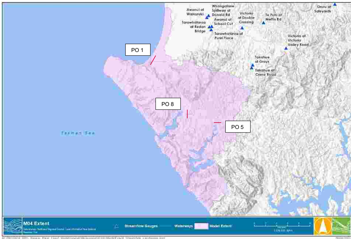
FIGURE 5-1 AVAILABLE STREAMFLOW GAUGES WITHIN WHANGAPAE AHIPARA CATCHMENT
