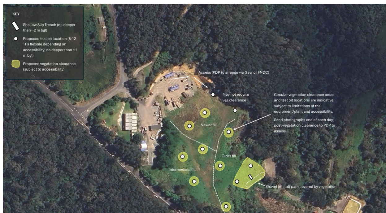
Figure 7 – Aerial View of the Russell Closed Landfill – The circles are the targeted trial pits for the cap investigation.
