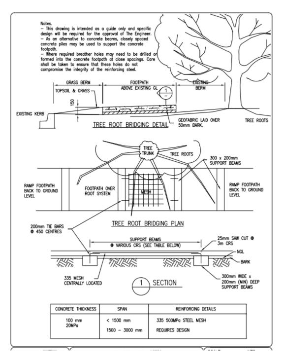
Fig 4 – Tree root bridging detail from Auckland Transport's Code of Practice 2008/0622.
