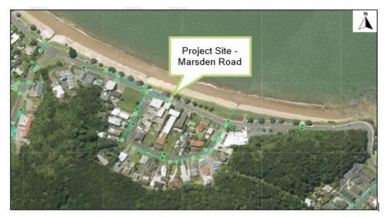
Figure 3: Existing Pit and Pipe network in green (Source: FNDC SW GIS Map)
