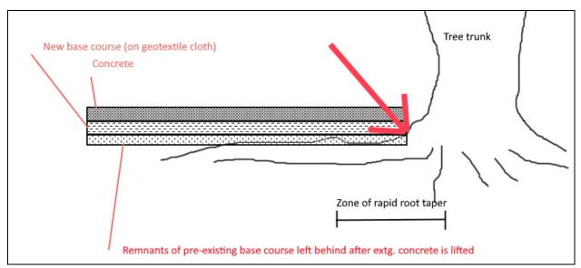
Fig 3 – Schematic of the relationship between a path and tree roots. The tree roots are relatively shallow and tend to invade the base course under paths. It is very important to avoid any significant cut in the vicinity of the red arrow, as this could cause direct damage to the roots. If the path is too close to the tree at this point, root action will lift the path.
