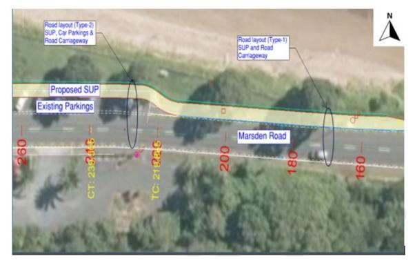
Figure 5: Proposed Road Layout (SUP, PARKING AND ROAD CARRIAGEWAY)
