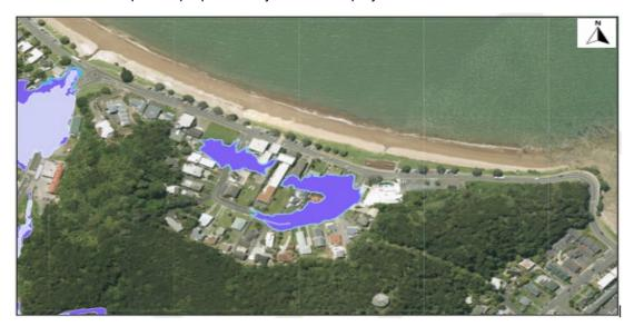
Figure 4: 1% AEP Flood plain (Source: FNDC (Flood modelling\_GHD, 2007))
