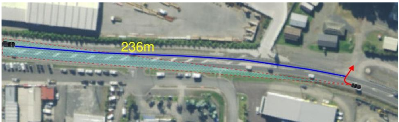
Figure 8: Available MGSD for vehicle on Northbound SH10 making right turn into the site.
