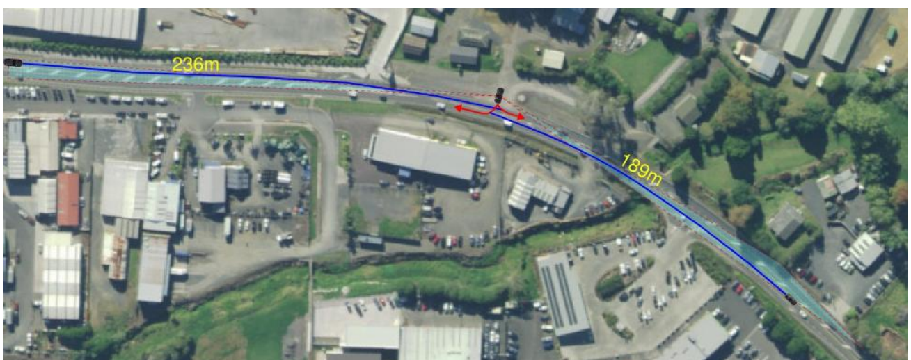
Figure 10: Available MGSD for vehicle at the access point turning right and left onto the SH10.
