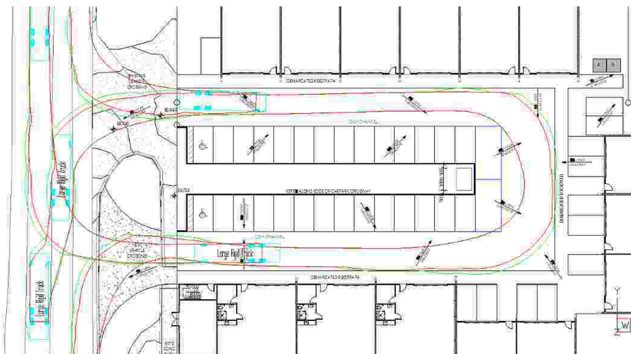
Figure 7: Large rigid truck tracking at the site's proposed separated entry and exit vehicle crossings
