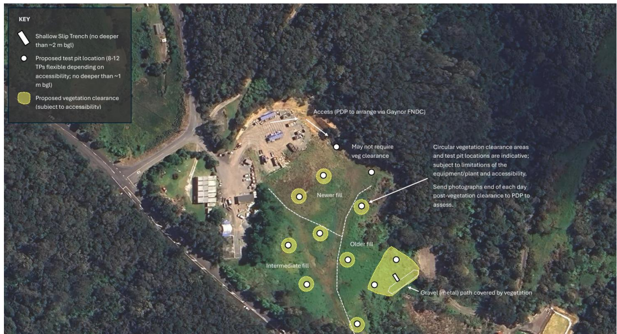
Figure 11 - Russell Closed Landfill: Locations of the investigation plots used to assess the condition and performance of the landfill cap.
