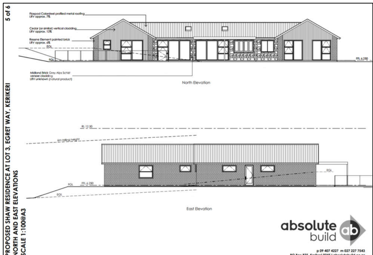
Figure 2. Elevations showing the proposed dwelling with existing/proposed ground profiles.
