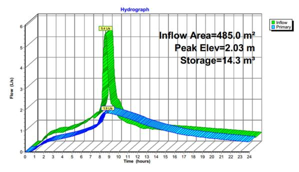
Figure 2: 1 x 15,000L Tank Attenuation Hydrograph
