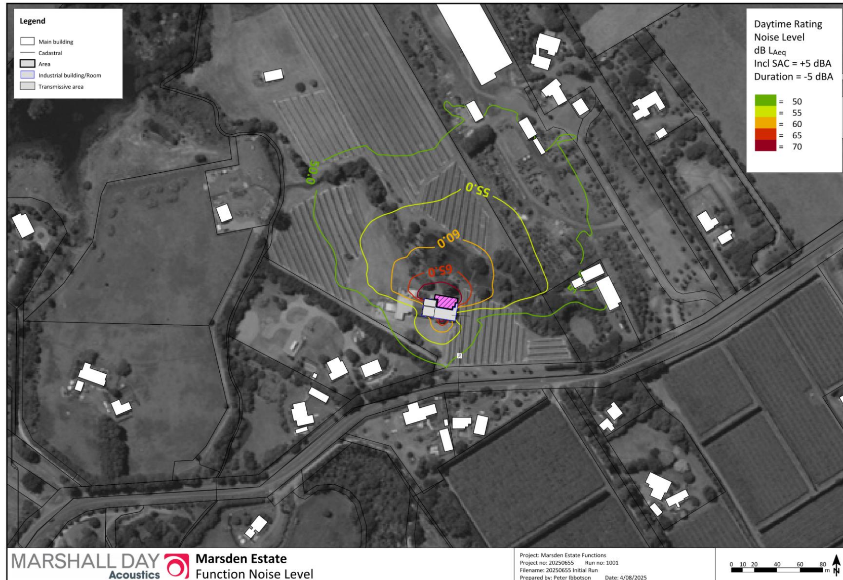
Figure 3: Grid Noise Map – Daytime Rating Noise Level – Function Room Doors Open, entry doors open at times
