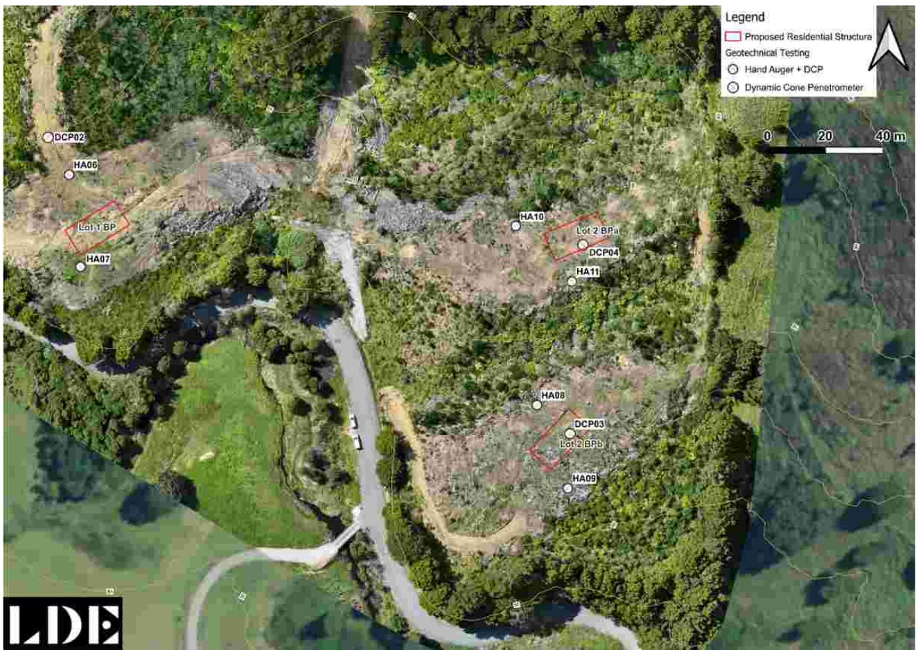
Figure 7: Geotechnical investigation plan.
