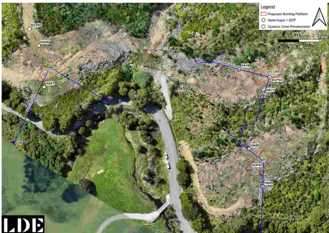
Figure 8: Cross section locations shown as blue lines. BP A is Building Platform A, BP B Building Platform B.
