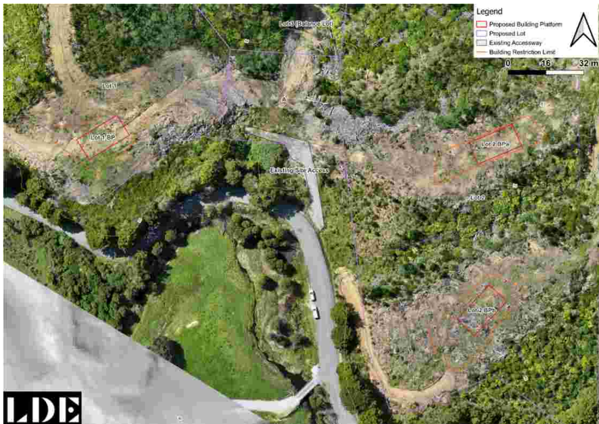
Figure 9: Building Restriction Limits, shown in orange, for each of the proposed building platforms, shown in red.
