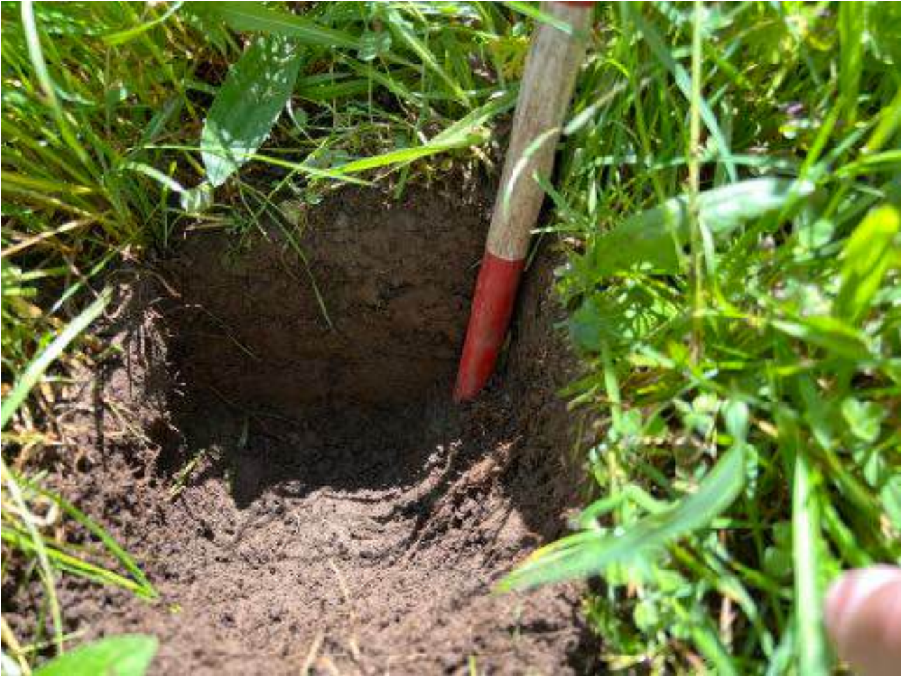
Figure 38. Detail of Test Pit 3 (within footprint of proposed stormwater infrastructure)
