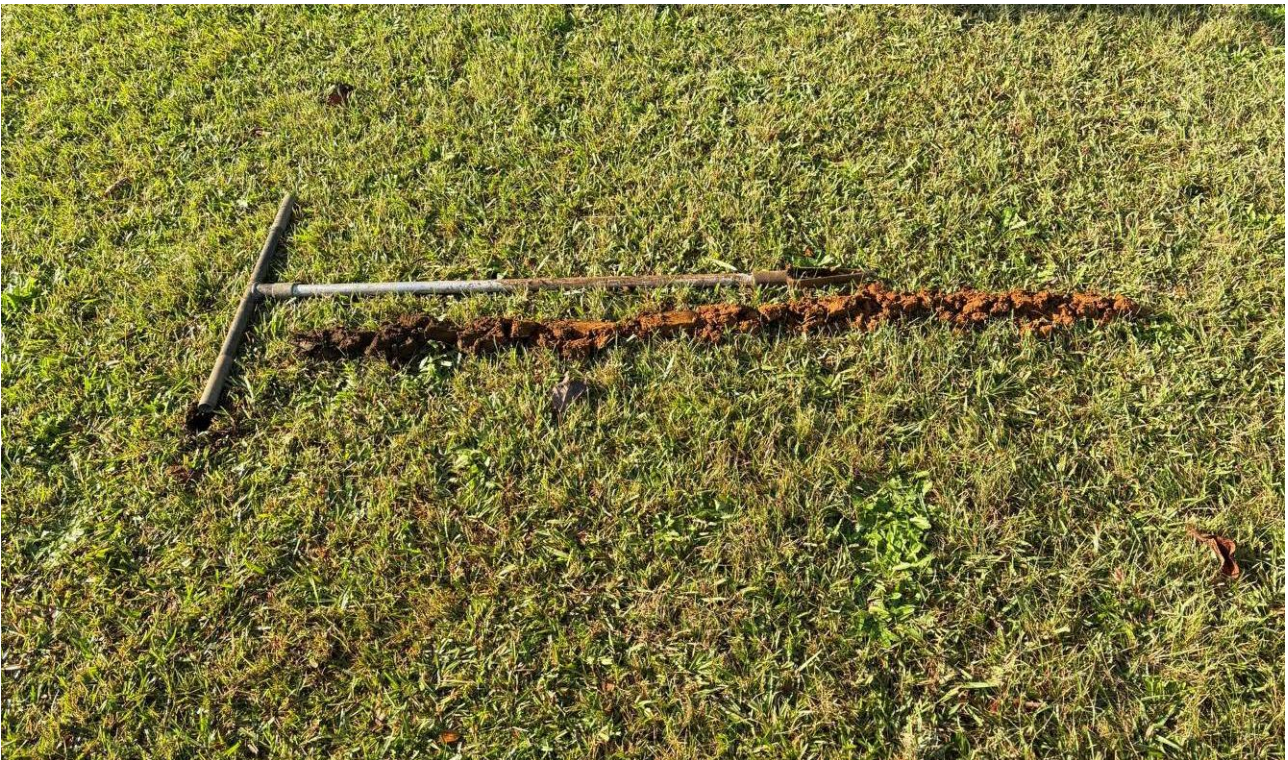
Photograph 2: 1.2m Deep bore showing soil layers. 200mm of topsoil followed by friable, silty clay.
