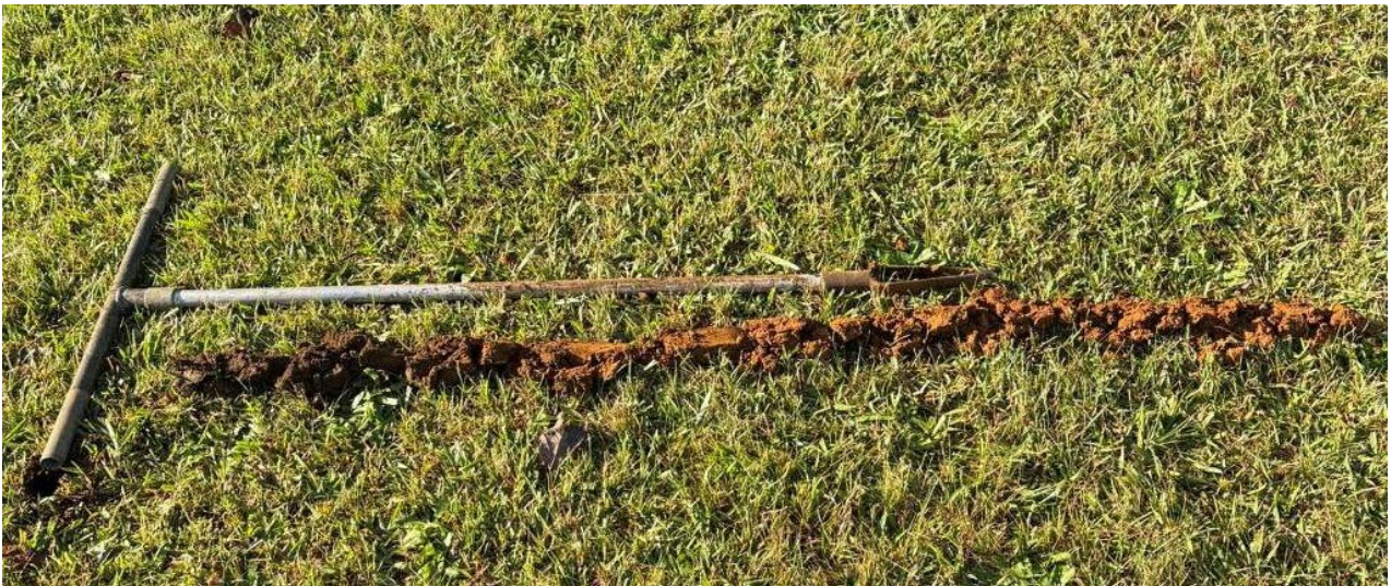
Photograph 2: Borehole showing 200mm of category 4, slightly moist, brown topsoil followed by category 4, slightly moist, brownish orange, friable, silty clay loam.
