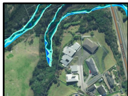
Figure 13: NRC Hazard Maps showing flooding extent around Waimamaku Stream.
