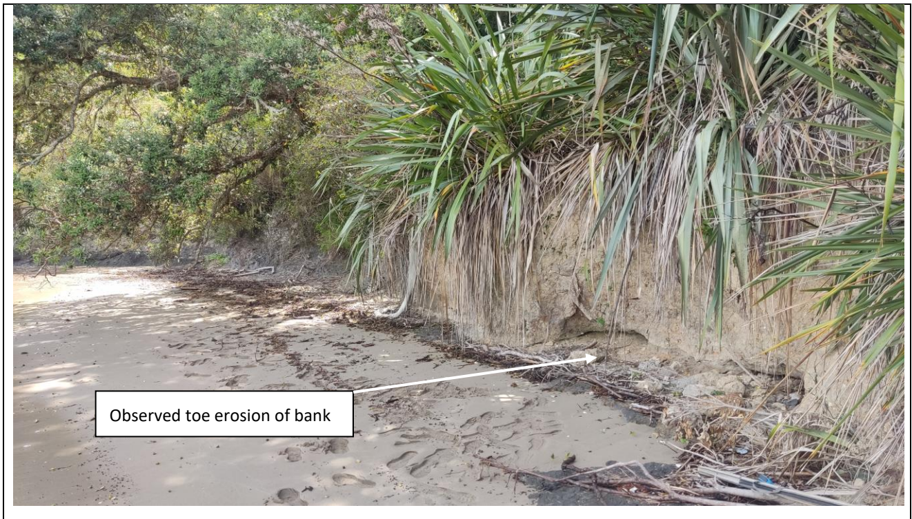
Figure 6 - Observed toe erosion of bank
