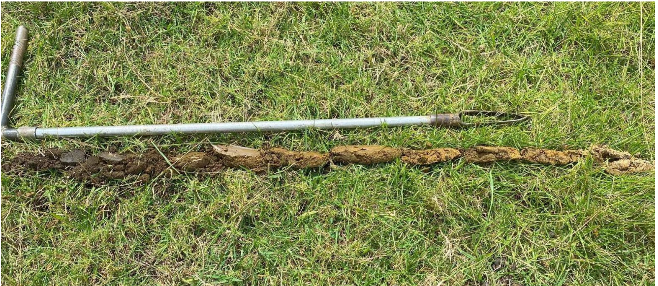
Photograph 2: Borehole showing 200mm of category 4, slightly moist, brown topsoil followed by category 6, slightly moist, orangey brown, silty clay to a depth of 1000mm. From 1000-1200mm soils became category 6, slightly moist, yellowish white, silty clay. The soils became siltier in the final 200mm.
