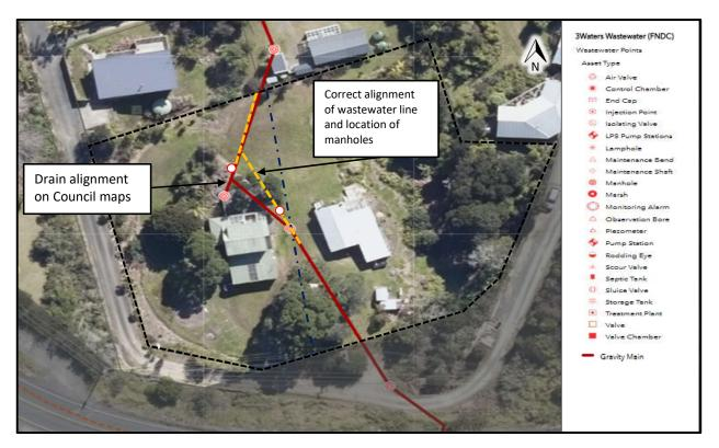
Figure 4: Existing wastewater network (Source: FNDC Water Services GIS service).
