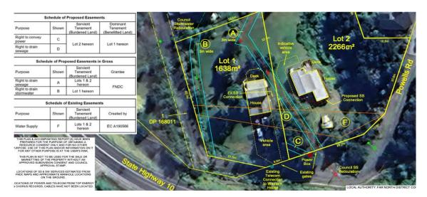
*Figure 12 : Western Dwelling and Easement Location <u>Source</u> Sapphire Surveyors Concept Plan*
