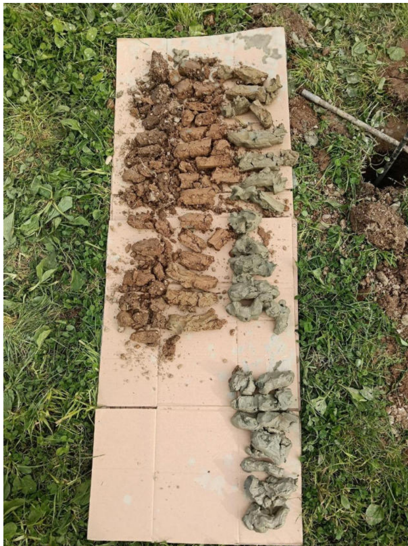
Figure 1: Hand auger samples taken from AH3 down to 3.90m bgl
