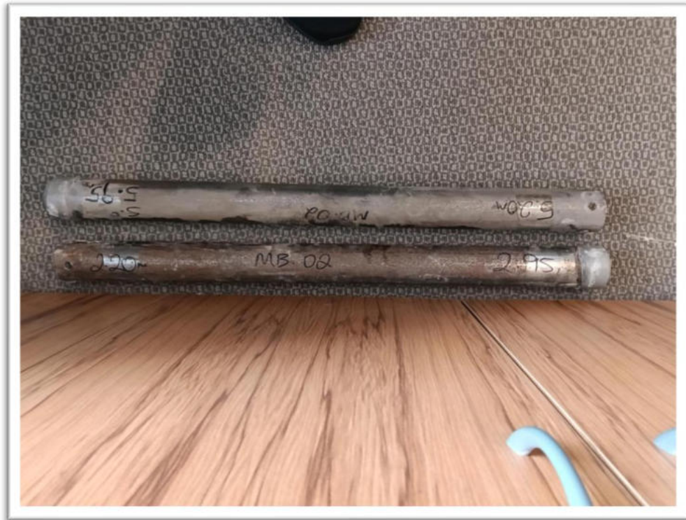
Photo 14: Push tube samples
