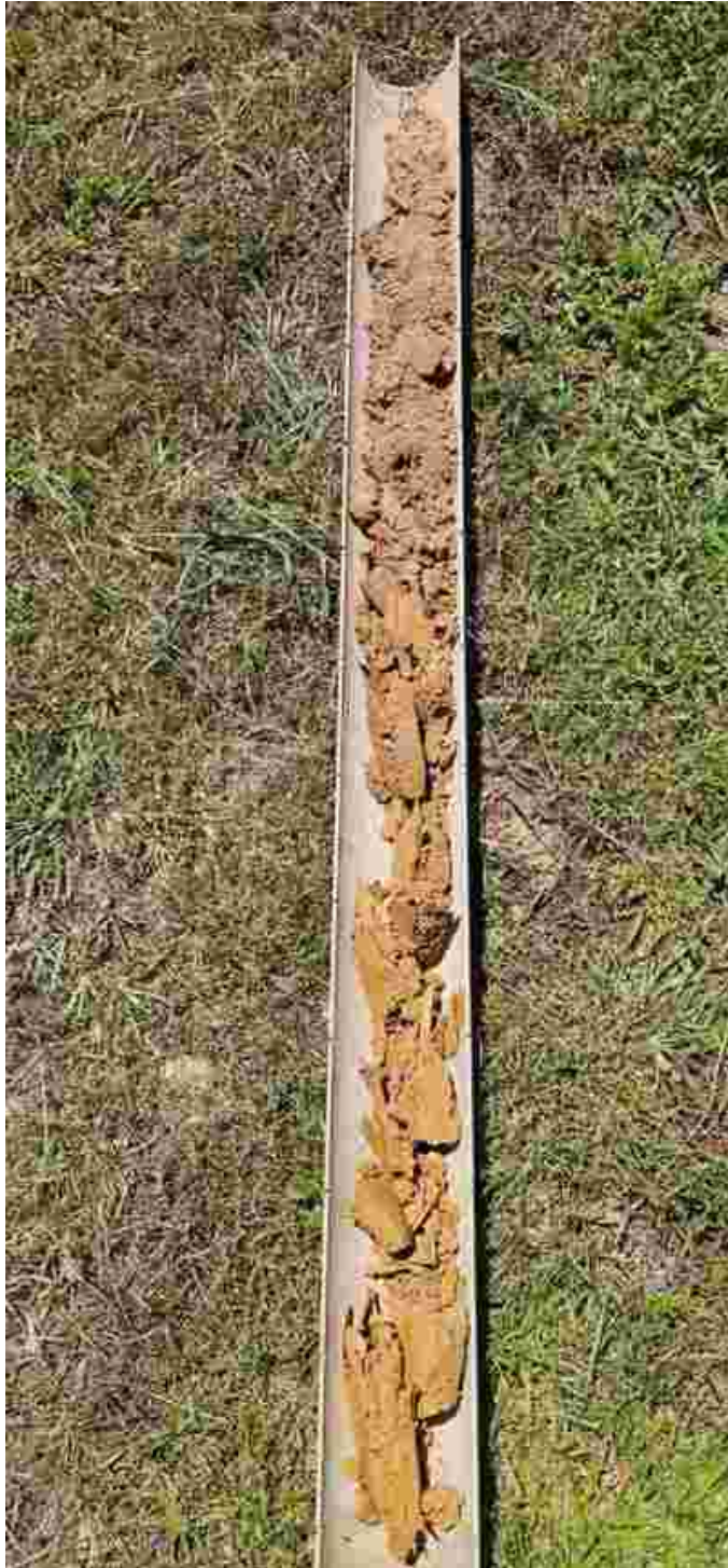
100mm layer of silty topsoil overlying silty clays Class 5, (as per AS/NZS 1547:2012 Table E1)
