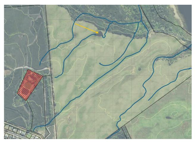
Figure 1: The wastewater treatment plant (red cross hatching), 5m contours (light yellow) and approximate surface (and near surface) water flows in dark blue. The yellow arrow points to the small pond where water quality samples have been taken. Rotokawau Lake (west) is just visible in the top right hand corner.
