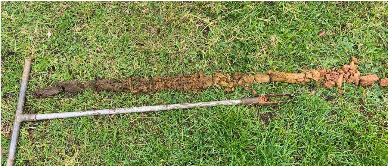
Photograph 4: BH2 taken on proposed Lot 3 showing 200mm of category 4, slightly moist, brown topsoil followed by category 4, slightly moist, silty clay loam with gravel to a depth of 500mm. From 500-700mm, a layer of category 6, slightly moist, orange clay was present. Soil from 700-1200mm became category 5, slightly moist, reddish orange, silty clay.
