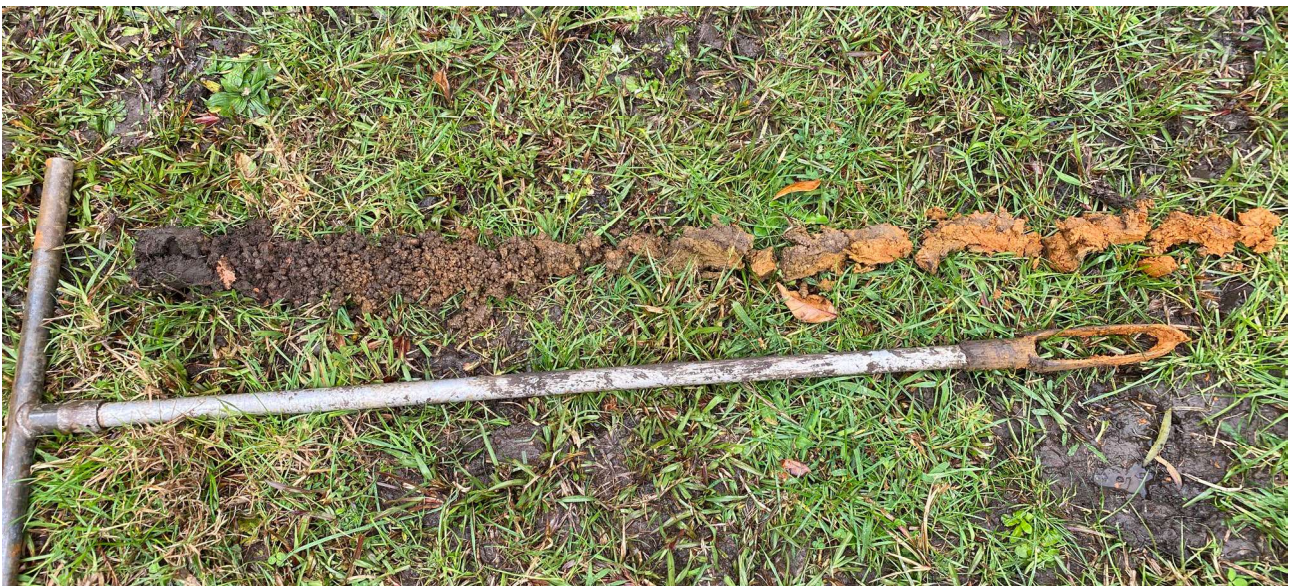
Photograph 3: BH1 taken on proposed Lot 2 showing 100mm of category 4, slightly moist, gravelly topsoil followed by category 4, slightly moist, brown, silty clay loam with gravel to a depth of 400mm. From 400-500mm, a layer of category 5, slightly moist, brown, silty clay was present. Soil from 500-1200mm became category 5, slightly moist, orange, silty clay.
